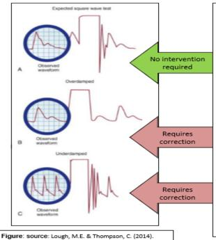
The normal dynamic response shows a square test waveform with one or two oscillations before returning to the baseline, this can be referred to as **optimally damped**.
